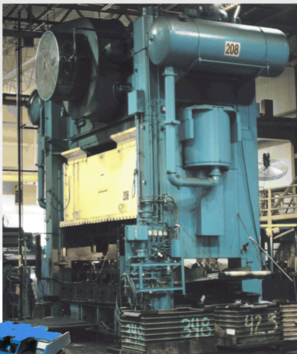
Installation of an 800 ton press on SVS Viscous Damped Spring Isolators.
